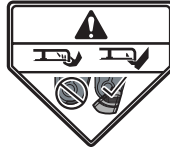
Warning! Keep away from the discharge deck, do not use without deflector or grass catcher
